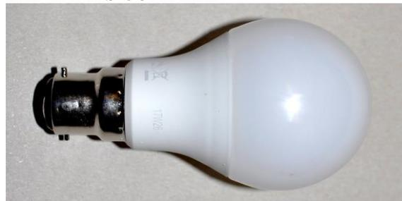
Peter Ireland has taken apart an LED lamp bulb (plastic), which showed a complex miniature electronics circuit board inside, obviously converting AC to DC, see pictures. The lamp, a 9 watt with 10 LED's, claiming that it is equivalent to a 60watt filament bulb and would last 20,000 hours. This one had failed after only a short use and was probably due to one of the component's failure!
